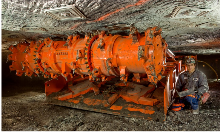
Joy 14CM Continuous Miner with Total Machine Power 805 HP in 58" Coal Seam in 2016
