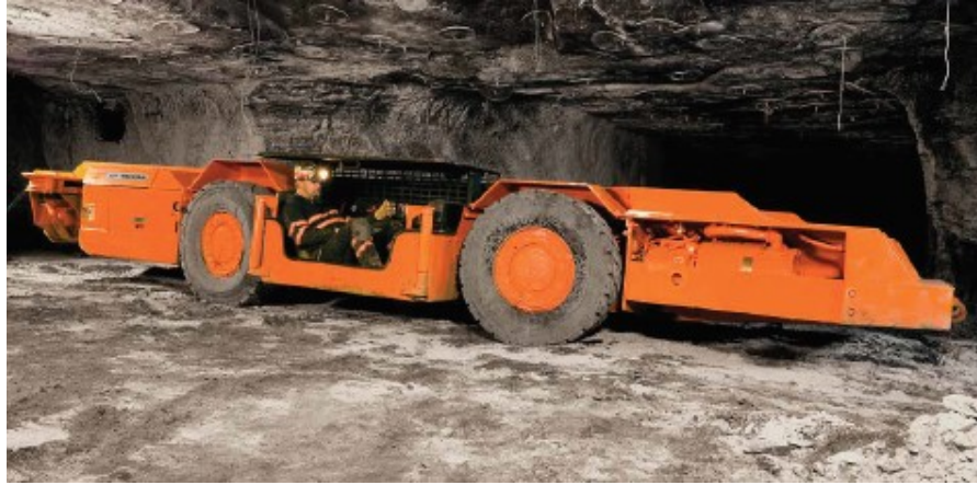
Joy 10SC32 Shuttle Car with Optidrive AC Variable Frequency Drive System Rated Load Capacity 12 Tons
