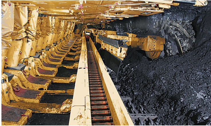
Caterpillar High Capacity Shearer Longwall System in 64" Seam
